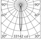
Luminous flux luminaire 1812 lm (EXTREME CUT OFF)
