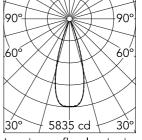
Luminous flux luminaire 1872 lm (EXTREME CUT OFF)
