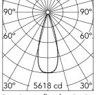
Luminous flux luminaire 1814 lm (EXTREME CUT OFF)
