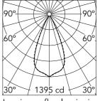
Luminous flux luminaire 735 lm (EXTREME CUT OFF)
