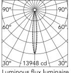
Luminous flux luminaire 773 lm (EXTREME CUT OFF)
