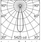
Luminous flux luminaire 793 lm (EXTREME CUT OFF)
