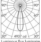
Luminous flux luminaire 738 lm (EXTREME CUT OFF)
