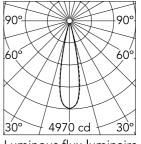
Luminous flux luminaire 744 lm (EXTREME CUT OFF)
