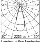
Luminous flux luminaire 732 lm (EXTREME CUT OFF)
