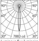
Luminous flux luminaire 437 lm (EXTREME CUT OFF)
