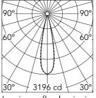
Luminous flux luminaire 475 lm (EXTREME CUT OFF)
