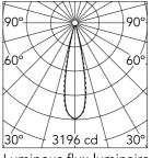
Luminous flux luminaire 475 lm (EXTREME CUT OFF)
