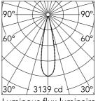
Luminous flux luminaire 470 lm (EXTREME CUT OFF)
