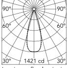
Luminous flux luminaire 455 lm (EXTREME CUT OFF)
