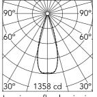
Luminous flux luminaire 441 lm (EXTREME CUT OFF)
