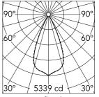
Luminous flux luminaire 2815 lm (EXTREME CUT OFF)
