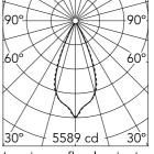
Luminous flux luminaire 2681 lm (EXTREME CUT OFF)
