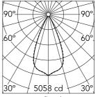
Luminous flux luminaire 2666 lm (EXTREME CUT OFF)
