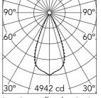
Luminous flux luminaire 2652 lm (EXTREME CUT OFF)
