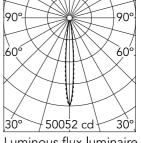
Luminous flux luminaire 2773 lm (EXTREME CUT OFF)
