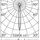
Luminous flux luminaire 2876 lm (EXTREME CUT OFF)
