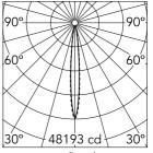
Luminous flux luminaire 2736 lm (EXTREME CUT OFF)
