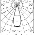
Luminous flux luminaire 2880 lm (EXTREME CUT OFF)
