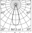
Luminous flux luminaire 2755 lm (EXTREME CUT OFF)
