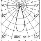
Luminous flux luminaire 2836 lm (EXTREME CUT OFF)
