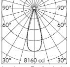
Luminous flux luminaire 2610 lm (EXTREME CUT OFF)
