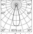
Luminous flux luminaire 2687 lm (EXTREME CUT OFF)
