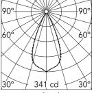
Luminous flux luminaire 183 lm (EXTREME CUT OFF)
