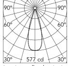
Luminous flux luminaire 185 lm (EXTREME CUT OFF)
