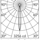
Luminous flux luminaire 184 lm (EXTREME CUT OFF)
