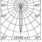
Luminous flux luminaire 1819 lm (EXTREME CUT OFF)
