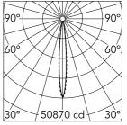
Luminous flux luminaire 2888 lm (EXTREME CUT OFF)
