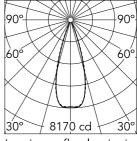
Luminous flux luminaire 2655 lm (EXTREME CUT OFF)
