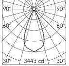
Luminous flux luminaire 1847 lm (EXTREME CUT OFF)
