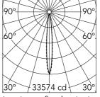
Luminous flux luminaire 1906 lm (EXTREME CUT OFF)
