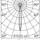
Luminous flux luminaire 1747 lm (EXTREME CUT OFF)
