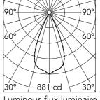
Luminous flux luminaire 464 lm (EXTREME CUT OFF)
