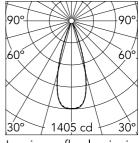
Luminous flux luminaire 454 lm (EXTREME CUT OFF)
