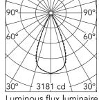
Luminous flux luminaire 1727 lm (EXTREME CUT OFF)
