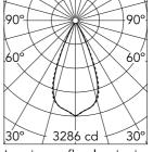
Luminous flux luminaire 1763 lm (EXTREME CUT OFF)
