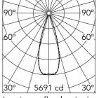
Luminous flux luminaire 1850 lm (EXTREME CUT OFF)
