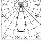
Luminous flux luminaire 1814 lm (EXTREME CUT OFF)
