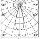
4 348 30° 5570 cd 30° 5 223 Luminous flux luminaire 1787 lm (EXTREME CUT OFF)
