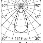
Luminous flux luminaire 716 lm (EXTREME CUT OFF)
