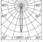
Luminous flux luminaire 785 lm (EXTREME CUT OFF)
