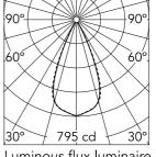
Luminous flux luminaire (EXTREME CUT OFF) 432 lm
