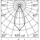
Luminous flux luminaire (EXTREME CUT OFF) 446 lm
