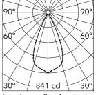
Luminous flux luminaire (EXTREME CUT OFF)
