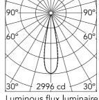
Luminous flux luminaire (EXTREME CUT OFF) 448 lm
