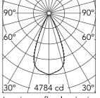
30° 4784 cd 30° Luminous flux luminaire 2597 lm (EXTREME CUT OFF)
